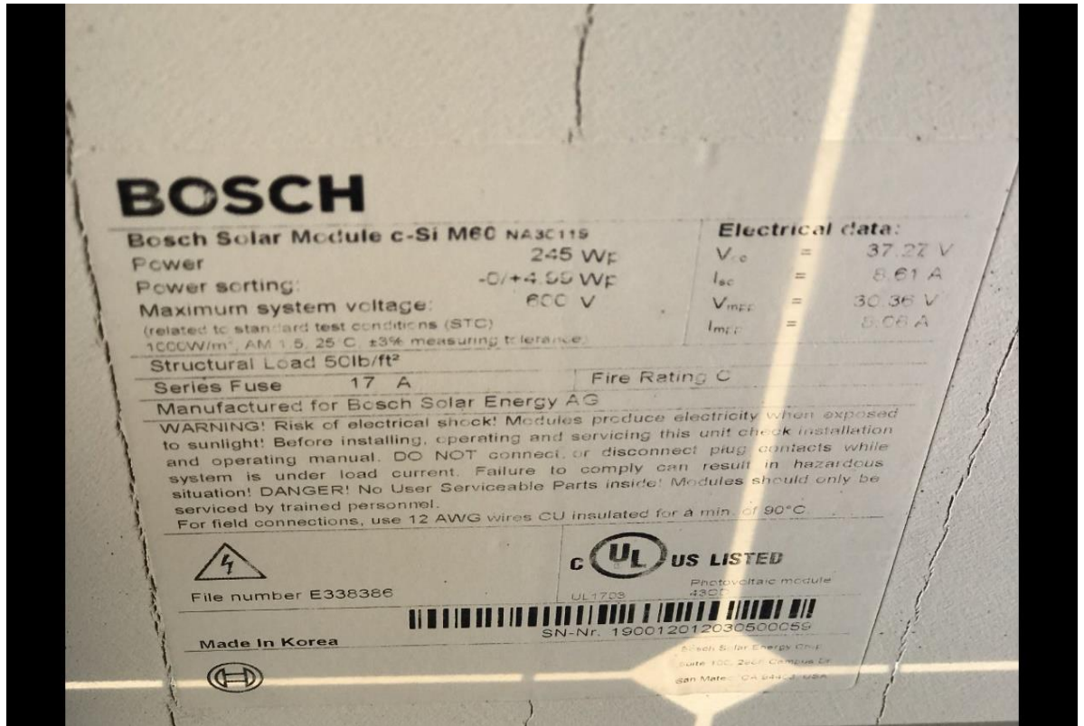
Label on the back side of a panel reflecting the Bosch Solar serial number identified as “c-Si M 60 NA30119”
